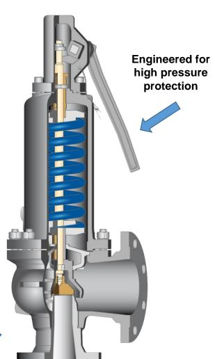
EPV 6303 high-pressure safety valve also for low temperatures
