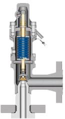
The Compact Safety Valve is installed in compressors and where ever medium must be relieved as effect of thermal exposure.
