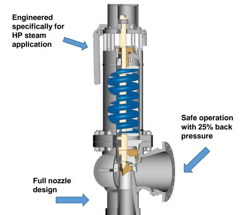
EPV 6106, high pressure steam safety valve with piston AK.
