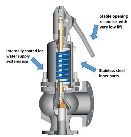
EPV 2321, our cast iron safety valve for basic applications
