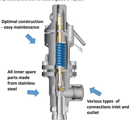
EPV C1329, the standard compact safety valve with threated connection
